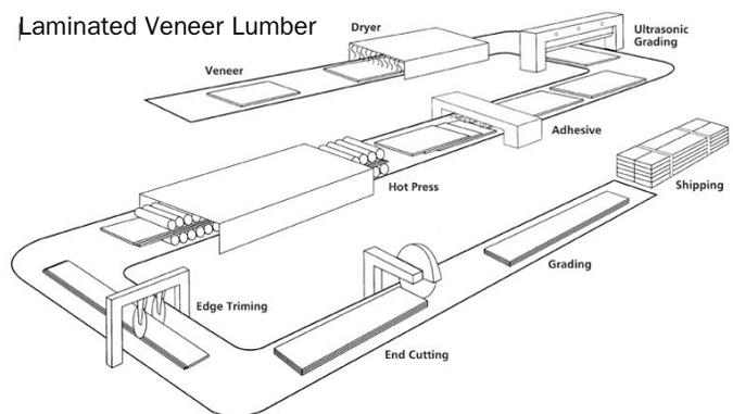
Structural composite lumber is available in a range of sizes and grades. The material typically undergoes final processing in a continuous or fixed press to form what is called a “billet” (for example: 4' wide x 60' long), which is then resawn into final product dimensions. SCL ranges in depths from 3<sup>1</sup>/<sub>2</sub>" to 18" and thicknesses up to 7".
