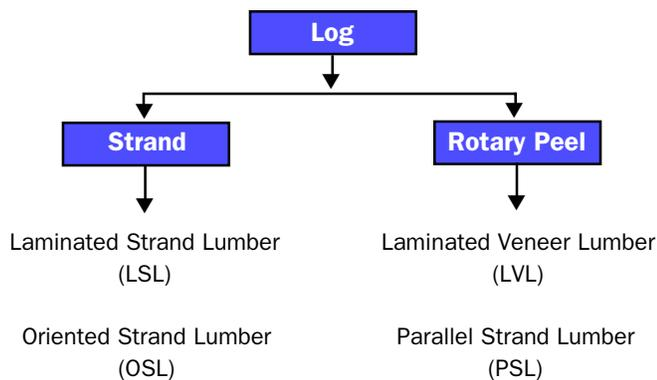
The manufacturing process for all SCL typically includes sorting and aligning the strands or veneer, applying adhesive, and pressing the material together under heat and pressure (Figures 4, 5, and 6). By redistributing natural defects, sorting for stiffness or density, and through quality control procedures, the resulting product is uniform.
