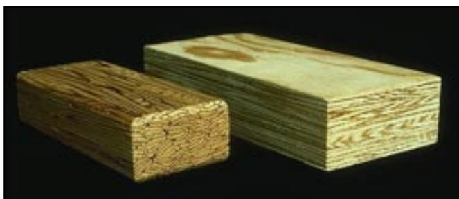
Parallel Strand Lumber (PSL) and Laminated Veneer Lumber (LVL) are two types of Structural Composite Lumber (SCL).
